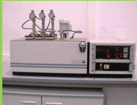
VST vicat softening temperature HDT heat deflection temperature
