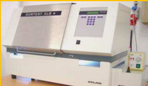
Weathering Xenon with water spray
